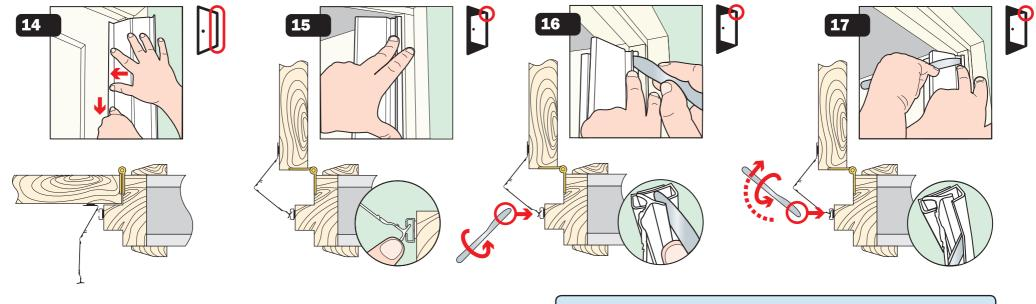
To temporarily unclip the shield for hinge access or door removal reverse stages 17 and 16 sliding knife downwards.
