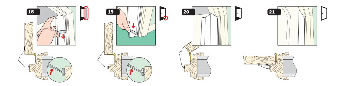
Extending Door Finger Protector<sup>®</sup> shield section for doors opening beyond the span of one hinge shield section
